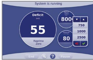
To adjust deficit limit setting, press the deficit limit 'Change' button, then select the preset deficit limits or use ▲▼ keys. Touch ✓.
