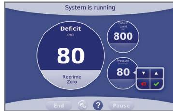
To adjust pressure setting, touch the pressure circle 'Change' button, then use the keys ▲▼ to set the pressure. Touch ✓. To start hysteroscopy, touch 'Run'.
