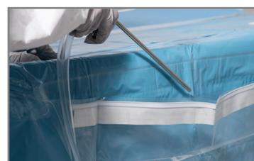
When the system is priming, fluid will run through FloPaks and all tubing.
