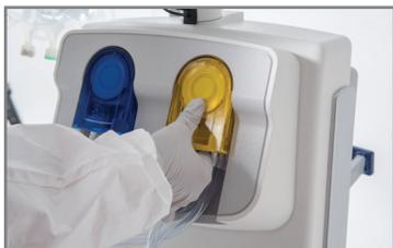
Insert yellow Out-FloPak as shown. Verify ✓ displays next to 'Install Out-FloPak' on the screen.
