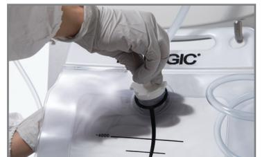
Connect (press on) Waste Bag outflow tubing to Waste Bag.
