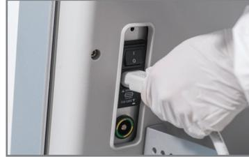
Plug in the power cord on back of console.
