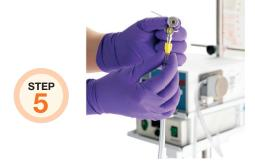
Twist the yellow luer-lock onto the scope outflow channel.
